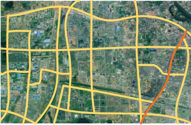
Fig. 8. Satellite aerial photography of tested area around the University of Science and Technology of China that is located in Anhui, China (from BaiduMap). The lines in the photo stand for the roads, and the orange one represents a viaduct. The network can be modeled as a digraph with 34 vertices and 108 arcs.
